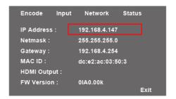
**3.2** Open the browser and input the IP address, e.g. 192.168.4.147, to access the login interface.
